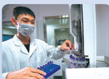
Polycyclic Aromatic Hydrocarbons (PAHs) Test on surface Coatings and Substrates
